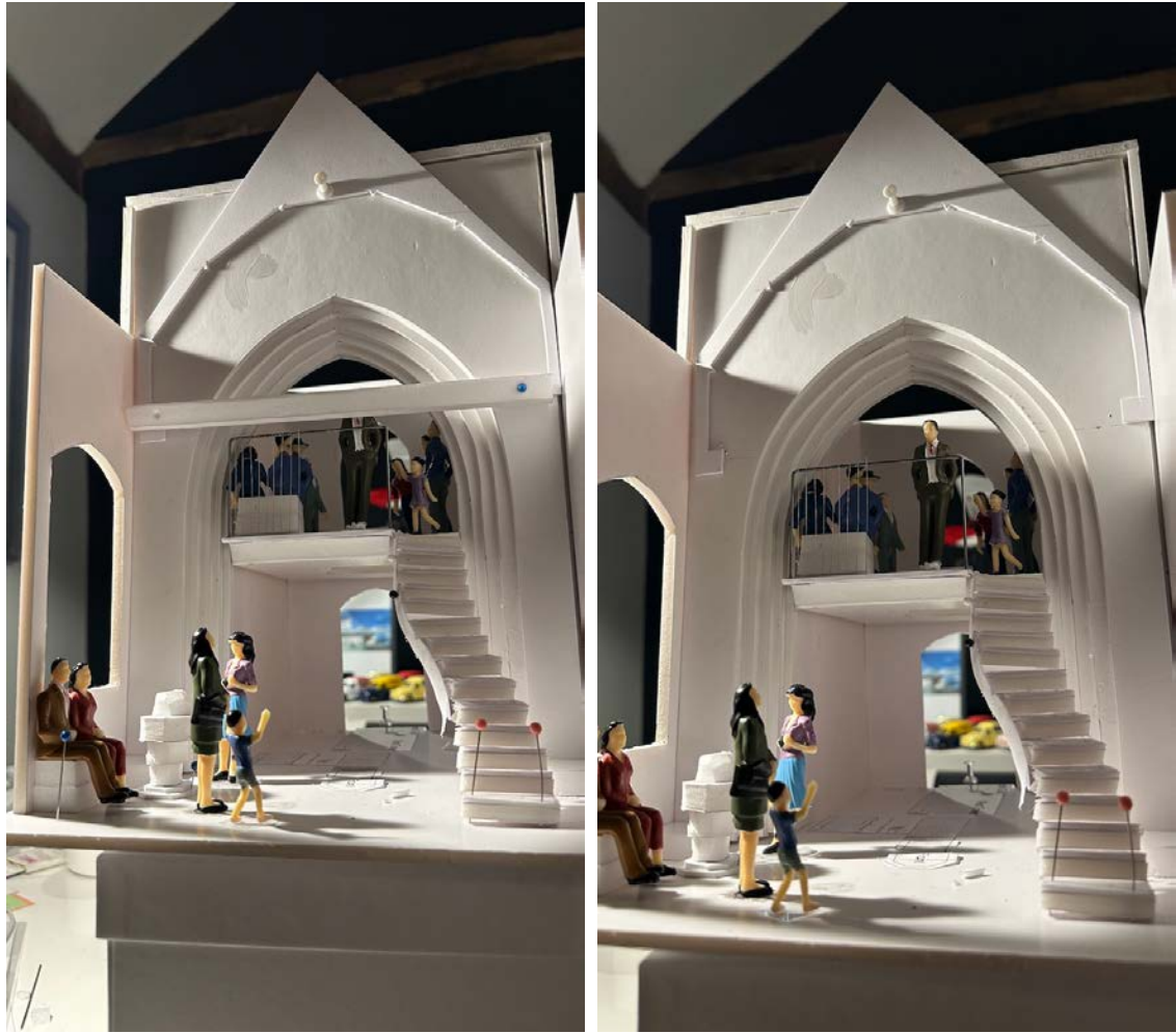
Photos of the working model showing the detrimental impact on the 15th century arch of the timber cross beam which is the subject of dendrochronological dating commissioned by Historic England. The view is looking west towards the proposed reinstatement of a bell-ringers floor in the west tower at St John the Baptist Church, Widford Listed Grade II*.
