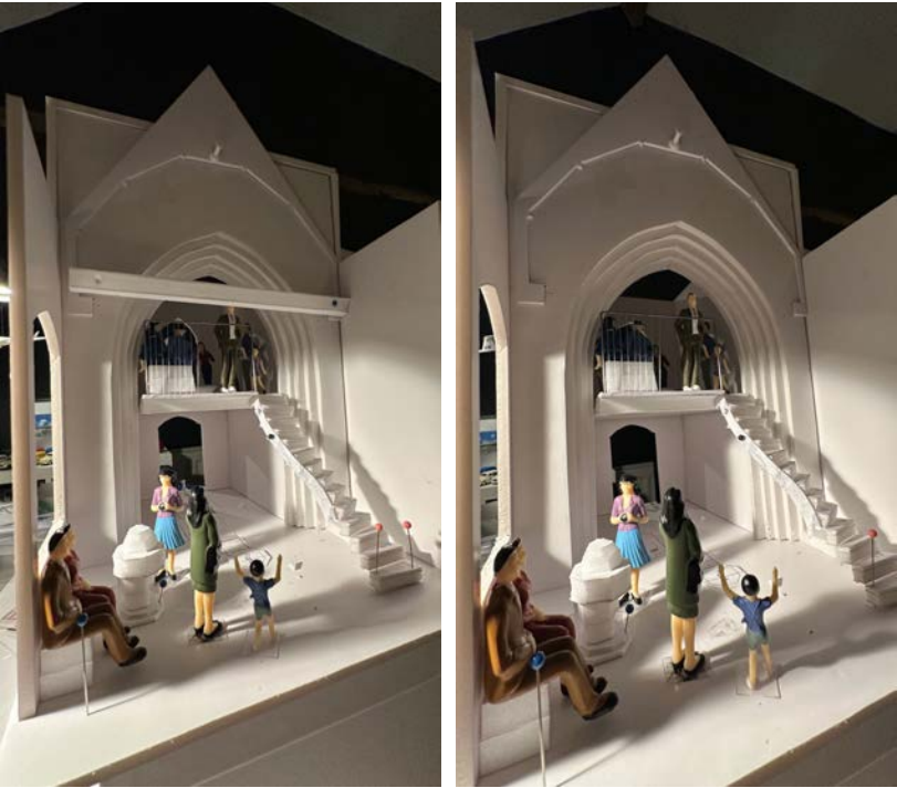
The arch and re-instatement of a bell-ringers' floor in the west tower at Widford is an opportunity to reveal the currently obscured 15th century stone arch and to make evident its relationship with the tall space of the belfry tower and the full height of the nave and its Wagon Roof
